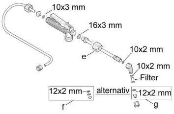
The spray tube is connected to the shut-off valve by means of screw cap (e).
