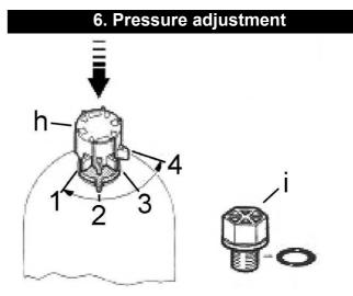
To regulate the output quantity/ droplet size, the spray pressure can be adjusted in steps from 1-4 bar.
