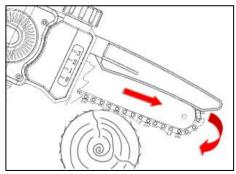
• When the guide plate is used for a bottom-up cut, the pushing direction of the saw is towards the operator.
