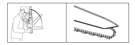
• When the bar is used for cutting from top to bottom, the tension direction of the saw is opposite to that of the operator.
