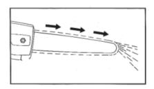
If no oil is flowing out, check if you have filled the tank.
