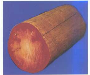
Boron diffusion shown via curcumin test after 4 months at approx. 85% humidity.
